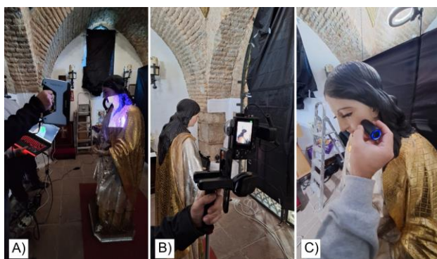
Figure 3. Data acquisition: a) SLS: EinScan Pro 2X; b) CRP: Sony Alpha 6100; c) colorimeter: NCS Colourpin-Pro.
