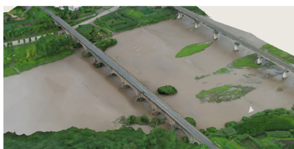
Figure 9. Tiled 3D model in Scene Layer Package (SLPK) format with RGB-based colouring from photogrammetry.
