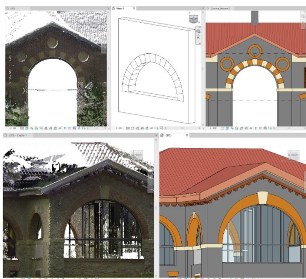
Figure 6: classification of arches as local family and modelling.
