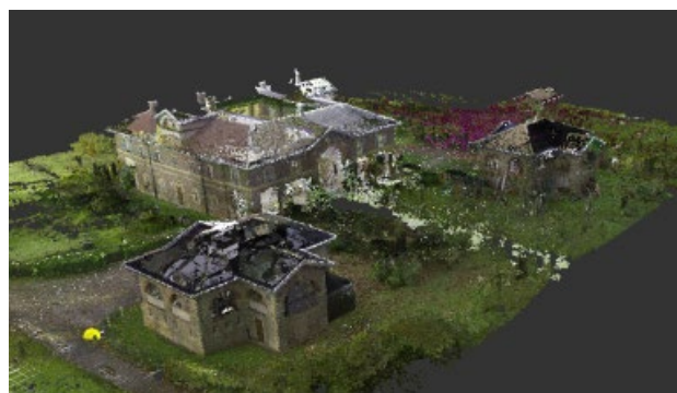
Figure 4. Point cloud from digital survey of the whole complex.
