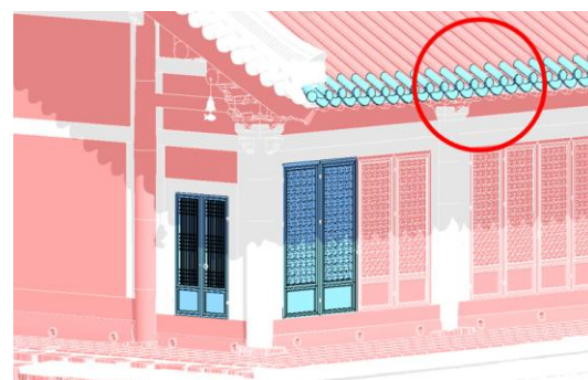
Figure 8. Restored ridge-end tiles ( Maksae giwa ) from the 1956 repair.
