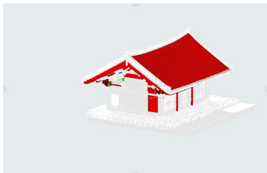
Figure 4. Repeatedly repaired components.
