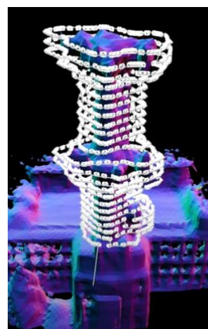
Figure 4. Example of the horizontal flightpath autonomously generated for a tower structure with Skydio 3D Scan
