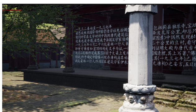
Figure 16. Foguang Temple Pillar within the Unreal Engine. 3D model of the pillar was digitised using close-range photogrammetry.
