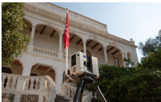
Figure 8. LiDAR scanning of Villa Portelli during fieldwork for the HERITALISE project.
