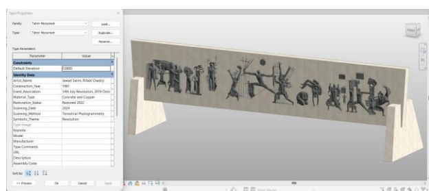
Figure 5. Family semantic parameters introduced in Revit.
