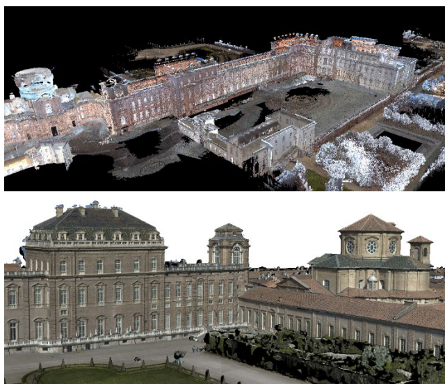
Figure 5. A portion of the registered MMS point clouds (above), 3D model of Reggia di Venaria generated via UAS (below)
