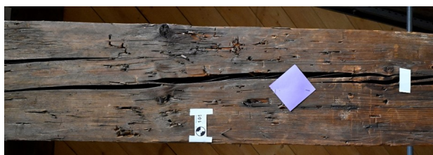
Figure 7. Examples of the real surface structure of historic timber with cracks, wooden knots and processing marks.
