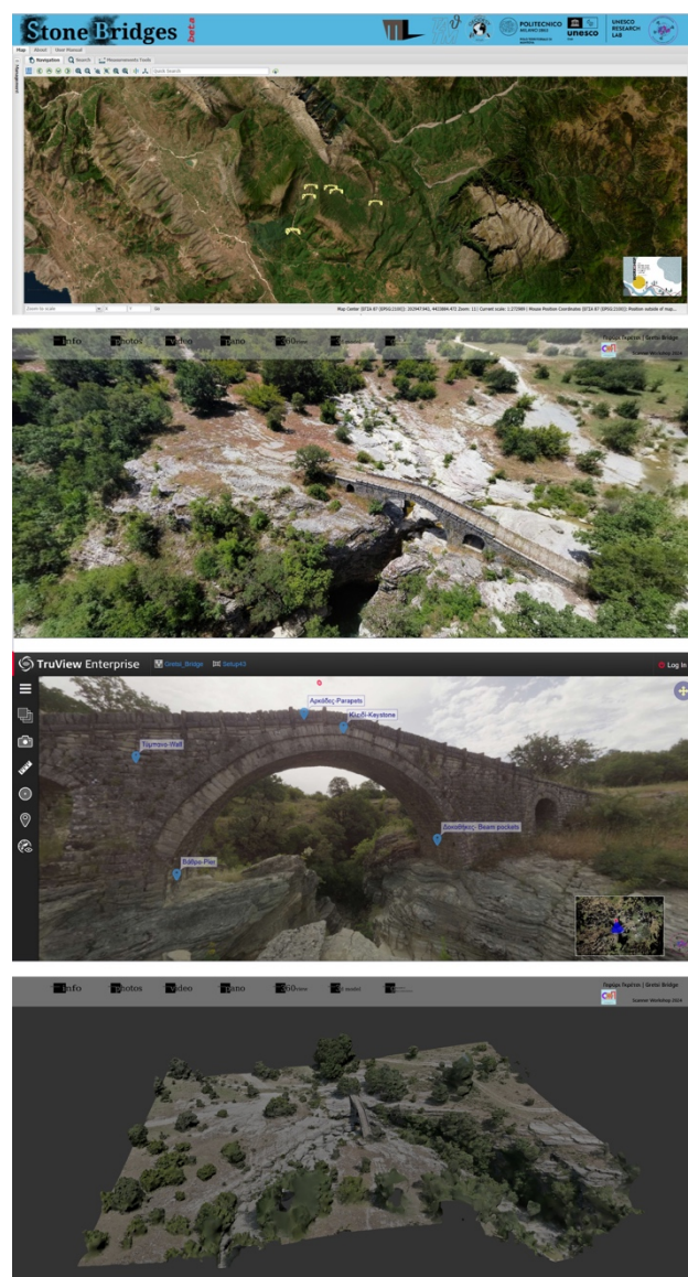
Figure 5. From top to bottom: a) screenshot of the geographic information system GIS with the identification of the surveyed area; b) 360-degree image exploration of Gretzi bridge; 3) Laser scanner data, explorable by the TrueView platform (Leica); virtual exploration of a single pointcloud.
