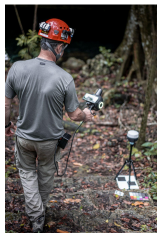
Figure 3. Collection of placed ground control point, color correction, and North arrow by the integrated multi-camera photogrammetry system (photo by M. Broen)
