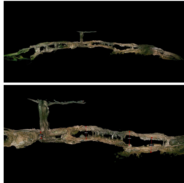
Figure 10. Cross Section of one of the vertical entrance complexes. Full model (top) shows the extent of the dry cave, from the entrance to the waterline. Partial subsections of the model (bottom) show the individual passages and the ability to take and display measurement data for later analysis.
