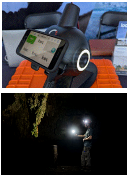
Figure 1. (top) Looq Integrated Multi-camera Photogrammetry system (photo courtesy of Looq). (bottom) D. Rissolo employs the Looq system in recording a partially submerged cave entrance (photo by M. Broen).
