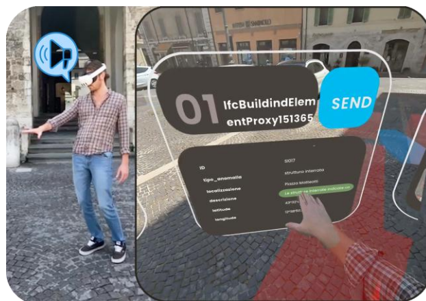
Figure 5. By setting the read/write mode it is possible to display and edit the information associated with the BIM platform. Based on the selected object, the related data is dynamically displayed within the interface. Each parameter can be edited through voice dictation. Once the editing process is completed, the updated content is first sent to Google Cloud and subsequently synchronized with the local BIM model.
