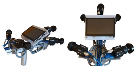
Figure 1. The ATOM-ANT3D fish-eye multi-camera portable mobile mapping system.
