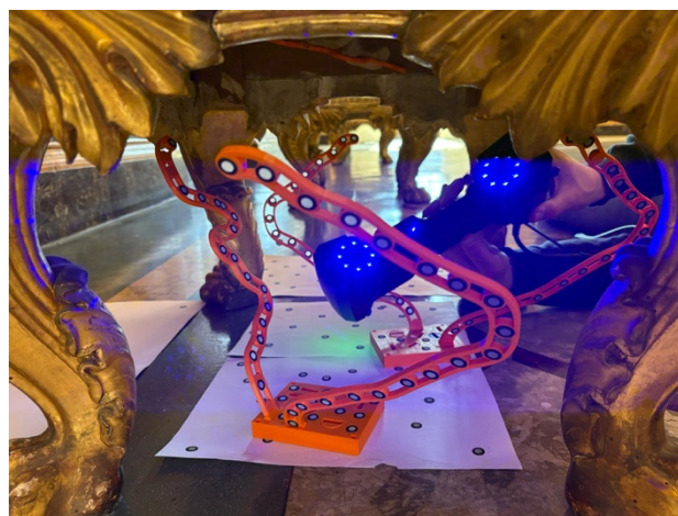
Figure 2. The strategy adopted to place markers for detailed survey of the artefacts in the Royal Palace of Caserta, using a handheld metrology-grade 3D scanner, Shining 3D FreeScan UE Pro.
