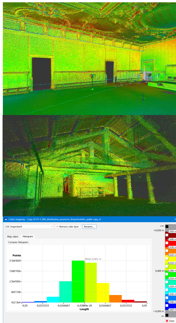
Figure 8. SLAM point cloud of the Grand Council Hall (on the top) and of a part of the attic (in the middle) colored by distance to the reference cloud. On the bottom the rainbow colour scale applied to the SLAM cloud, depicting its distance from the reference cloud. The inspection range was 5 cm.
