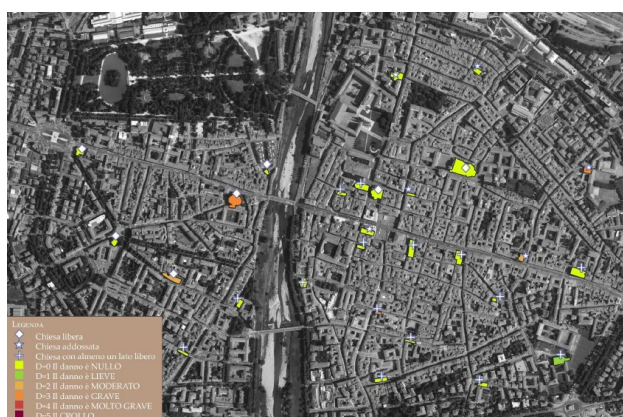
Figure 3. Example of GIS analysis investigating the correlation between the constructive features of Parma masonry churches and the level of damage for out-of-plane mechanisms caused by 1983 earthquake (Privitera, 2025).
