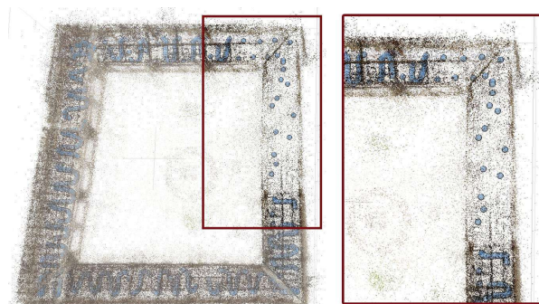
Figure 4. Without live feedback the operator accelerated subtly, leaving the last five metres with too few viewpoints to support dataset convergence.
