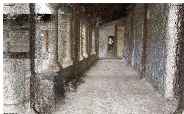
Figure 5. View of the point cloud following photogrammetric processing from 360-degree panoramas, in which it is possible to see the lack of data at areas not affected by the survey.
