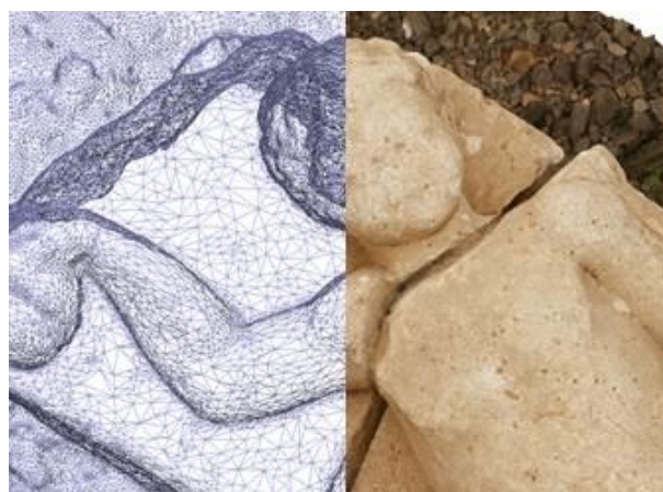
Figure 7. Detailed three-dimensional model of a sculpture of the cathedral, mesh (left) and texturized (right).
