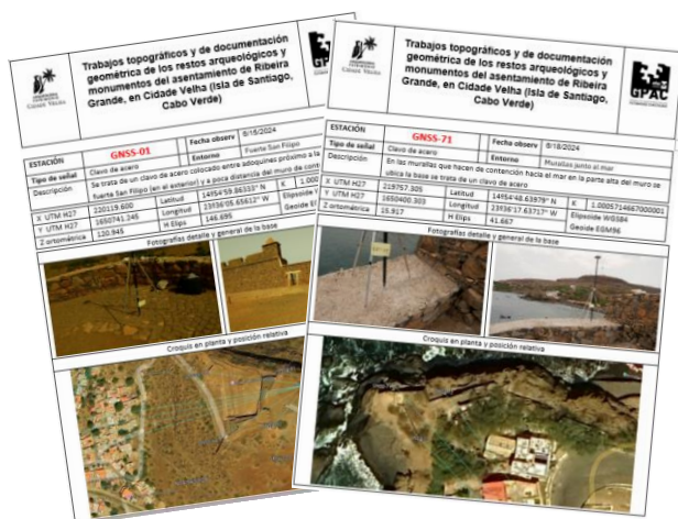
Figure 5. Examples of descriptive cards with the location and coordinates of the benchmarks of the topographic network.
