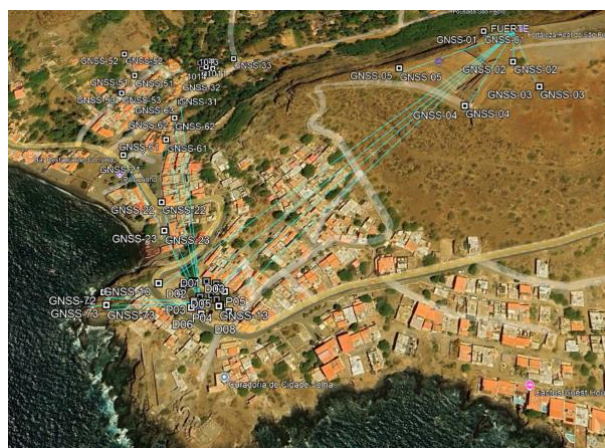
Figure 2. Reference network observed by GNSS, distributed for all the areas with historic remains.
