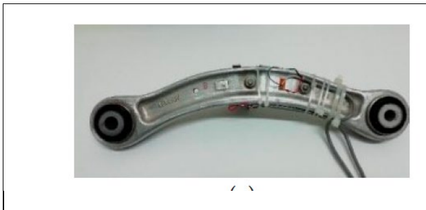
Figure 10. The placement of the sensor to calculate the stress and strain in laboratory on the part of the suspension.
