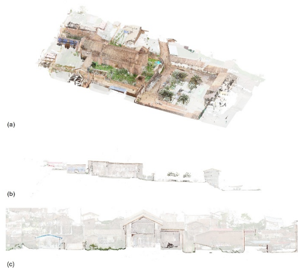
Figure 2. Views of the registered point cloud in (a) perspective view, (b) longitudinal view, and (c) lateral view.
