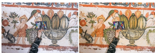
Figure 3. Unedited image (left) compared with white balanced and colour calibrated image for terrestrial photogrammetry (right).
