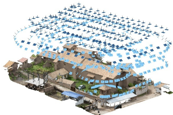
Figure 1. Camera positions of drone images captured with the Mavic 3 Pro.
