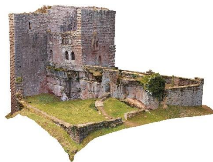
Figure 1. Mesh of the castle of Wasenbourg. Processing based on lasergrammetric and photogrammetric surveys.
