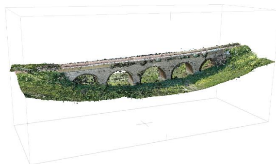
Figure 5. Dense point cloud obtained from the UAV survey after post-processing with Metashape.
