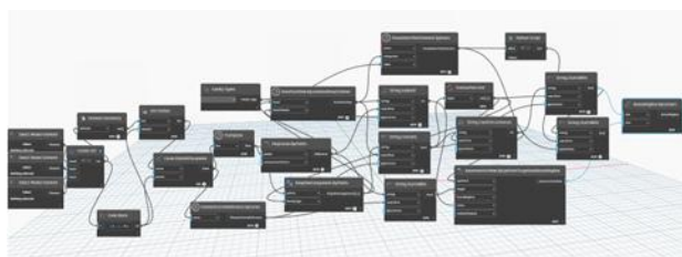
Figure 17. Dynamo node sequence for the generation of adaptive components in the BIM model.
