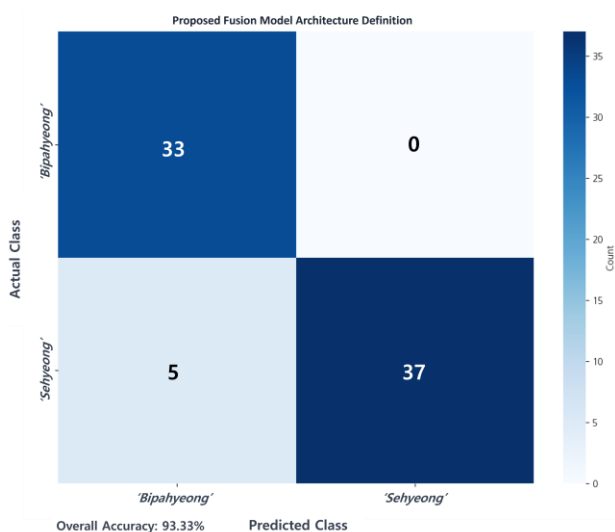
Figure 6. Confusion matrix evaluation results for the proposed fusion model.
