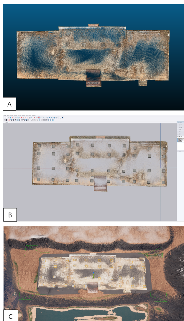
Figure 7. Point cloud capture and digital reconstruction of the archaeological remains of Hyeumwonji Building 1-2.
