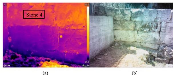
Figure 10. IRT image revealing thermal anomalies (a), Corresponding RGB image of the same section of the Wall 1 (b).
