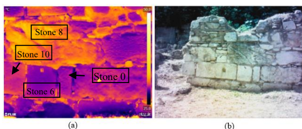
Figure 11. IRT image revealing thermal anomalies (a), Corresponding RGB image of the same section of the wall 2(b).
