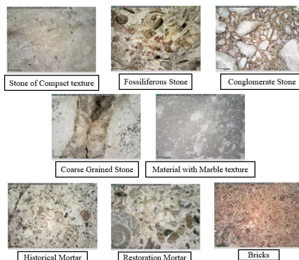
Figure 5. Digital microscopy images of the building materials.
