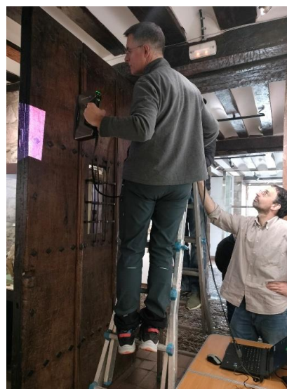
Figure 1. Three-dimensional recording (with a fringe-projection scanner) of the graffiti (and the surfaces where they are) on one of the doors of the museum.
