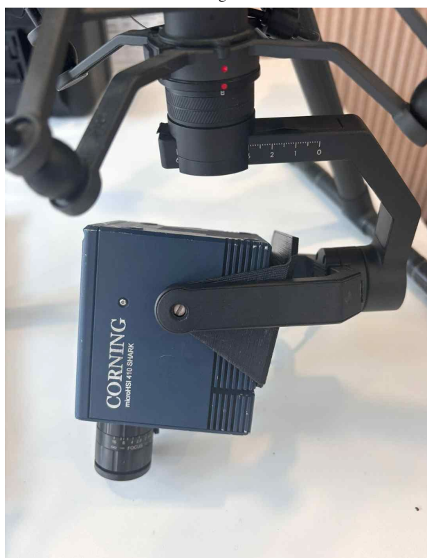
b. Precision 3-Axis gimbal system (improved design)
