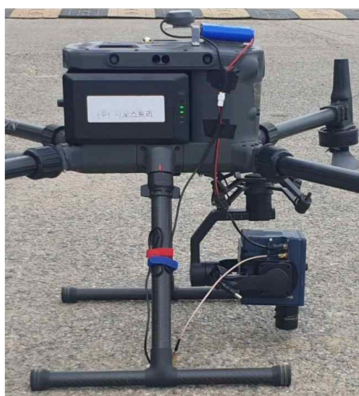
b. Power cable, Landing gear, External battery Installation
