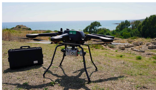
Figure 1. The RIEGL VUX-1UAV 22 aerial laser scanner and AceCore Noa drone platform we deployed to Kamarina and Heloros to capture the ALS data used in this study.
