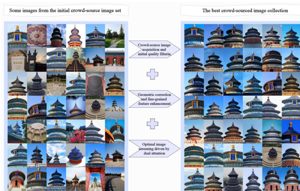
Figure 7. Schematic diagram of the crowd-source image optimization process: The initial image set contains original data of ancient buildings taken from multiple angles, with problems such as perspective distortion, occlusion, uneven lighting, and irrelevant images; the optimal image set processed by the method proposed in this study has significantly improved resolution and color consistency, and key components such as brackets and caissons are completely preserved. CBAM-EfficientNet effectively screens out target images and suppresses problems such as low quality and occlusion interference.
