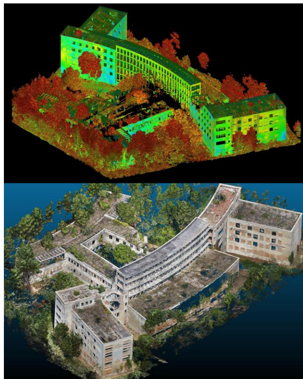
Figure 12. Views of the 3D point cloud and the model obtained through photomodelling (graphic elaboration by the authors).
