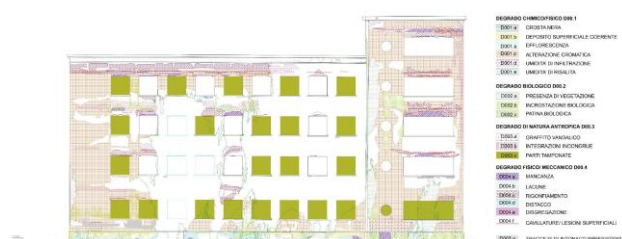
Figure 15. CAD mapping, with degradations represented in vector format for computational purposes (graphic elaboration by the authors).
