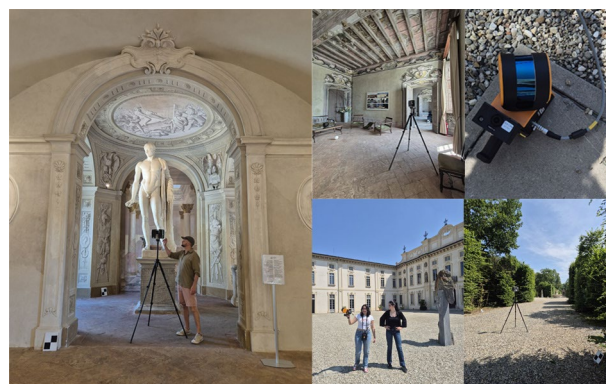
Figure 7. Laser scanning, topographic, and photogrammetric survey operations.
