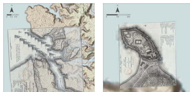
Figure 5. Archival maps (Figure 5) are georeferenced with DEM in GIS. The DEM illustrates present-day topography. Left: Profile of Vaghotan Creek. Right: Vijaydurg fort and land connection to the town. © Authors
