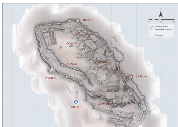
Figure 2. The layout and 3D photogrammetric model of Fort Vijaydurg is georeferenced with a Digital Elevation Model generated in ArcGIS. The map depicts location and assumed heights of the viewpoints considered for viewshed analysis. © Authors
