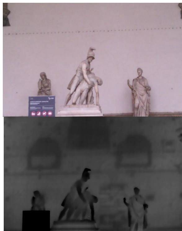
Figure 1. Photograph and corresponding thermographic image revealing structural makeup of wall behind the Loggia dei Lanzi.
