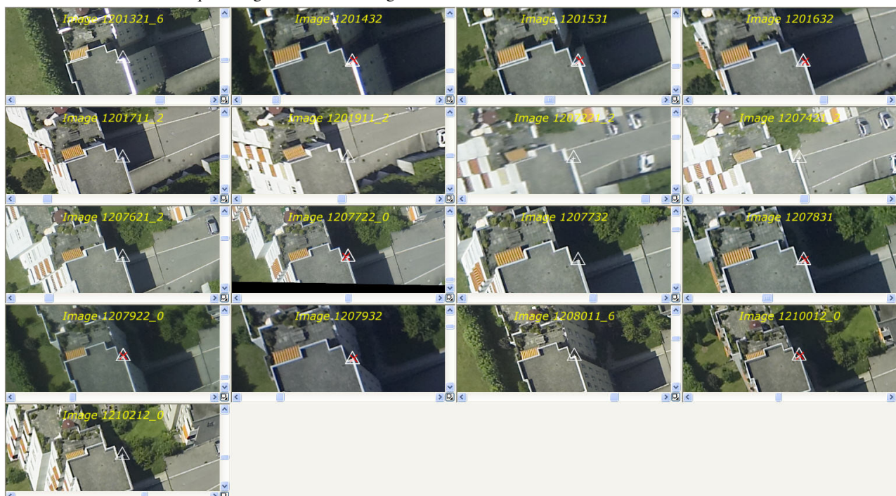
Figure 2: Manual Measurement of Tie Points in 17 Oblique Images with Match AT
