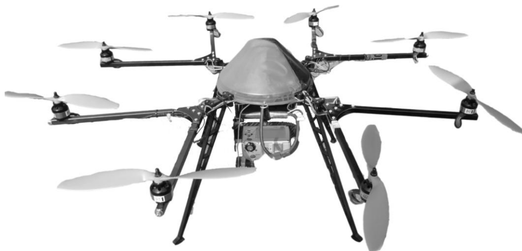
Figure 2. Mini-UAV MK-Okto by HiSystems GmbH (HiSystems GmbH, 2012) equipped with NEC F30 IS thermal imaging system
