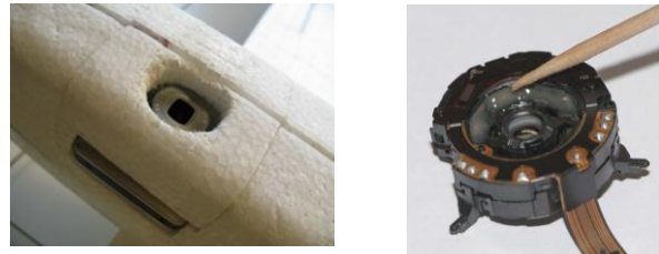
Figure 2: Used consumer camera mounted on UAV belly (left) and fixed lens element (right).
