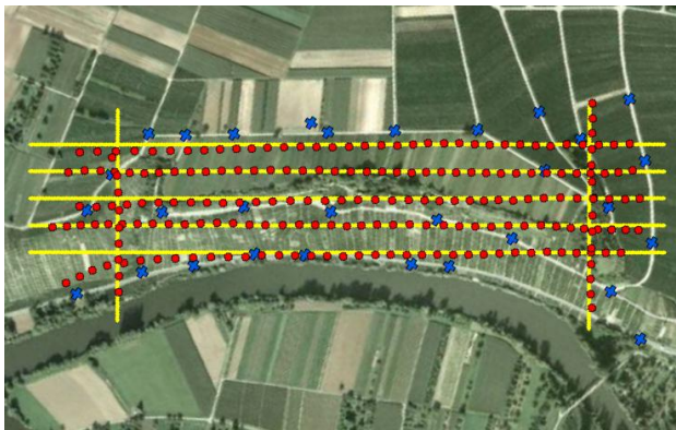
Figure 3: Test-site Vaihingen/Enz, with planned flight lines, camera stations from GPS measurement, and signalized points.
