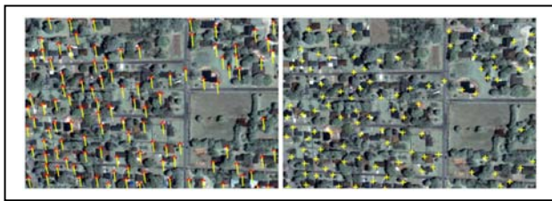
Figure 3. Corners in the first image are detected using Harris corner detector, and then Lucas-Kanade optical flow is applied to find corresponding feature points in the second image. Left image shows detected corners and optical flow vectors against the detected corners on the right image.
