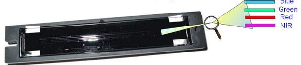
Figure 8: multi-spectral sensor
