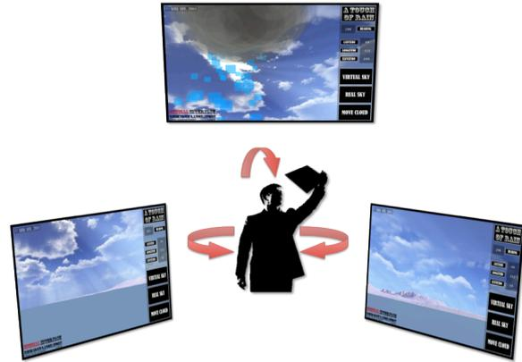
Figure 6. A situated virtual environment interface – using a location-aware, camera-equipped, sensor-enabled tablet to ‘look through’ a portal into a virtual world at the same scale as the real world. The user can move the tablet to look around at data visualizations of the space they are standing in.
