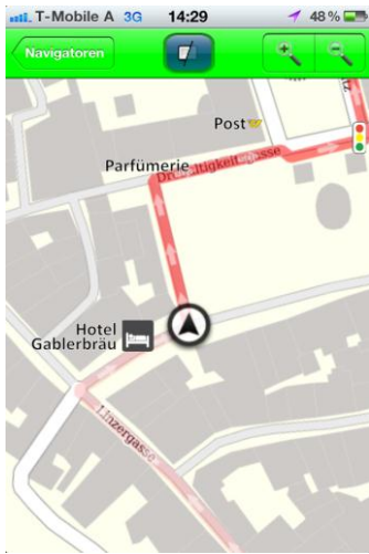
Figure 1. A screenshot of the map-based interface, with an egocentric view, distinction between the past and future paths, automatic adaptation to real-time location, zooming and panning functions, etc (© Salzburg Research, Map data: OpenStreetMap and Contributors, CC-BY-SA).
