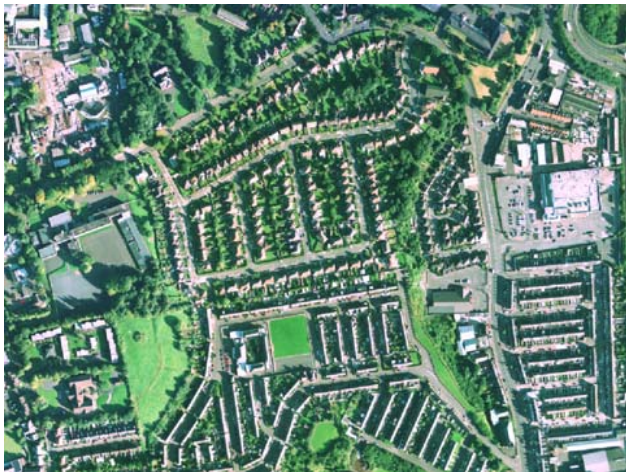
Figure 1a: Micro urban remote sensing. Digital aerial photography at a spatial resolution of 12 cm (Belfast, UK).
