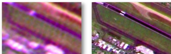
Figure 6 – TM images (3R4G2B), Goiânia Airport: Multispectral image (left) and hybrid image (right).
