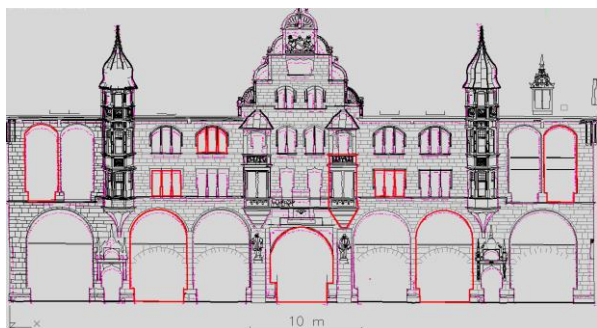
Figure 4. Restituted map (in black) with assessment contours (in red). Extracted contour points appear in magenta.
