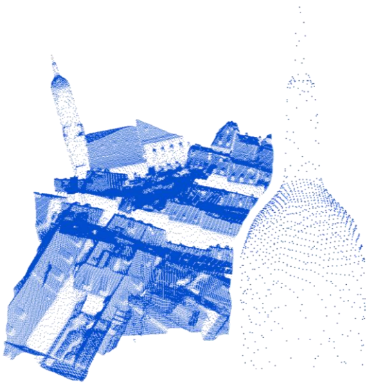
Figure 4. High resolution 3D point cloud generated by the dense matcher module of UltraMap
