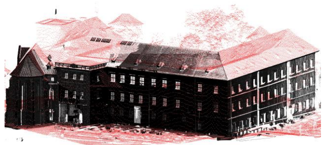
Figure 2. Example of the combined point cloud (part of terrestrial (black) and airborne (red) laser scanning data).
