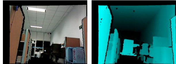
Figure 2: (left) RGB image and (right) depth information captured by an RGB-D camera. Black pixels in the right image have no depth value, mostly due to max distance, or surface material.
