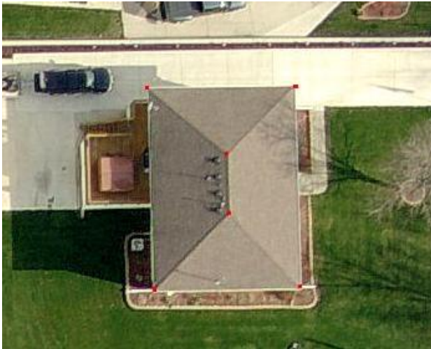
Figure 5. Match points of hip roof (red dots)
