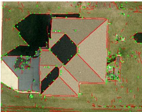
Figure 1. Extracted points (green) and edges (red)
