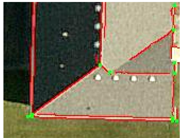
(a) Image edges before removal of gutters
