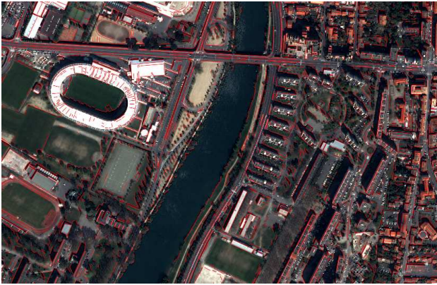
Figure 4. Example of Orfeo ToolBox algorithm results: Pan-sharpening and Line segment Detection on a Quickbird image of Toulouse, France.
