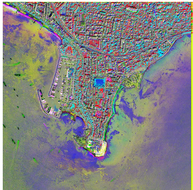
Figure 3. Example of Orfeo ToolBox algorithm results: MAD/MAF analysis (Nielsen et al., 2010) on a pair of 4 bands Worldview2 images of Cannes, France.
