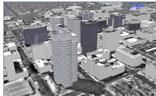
Fig. 1 3D city model from QuickBird images reconstructed by the CC-Modeler (Kocaman and others, 2006)
